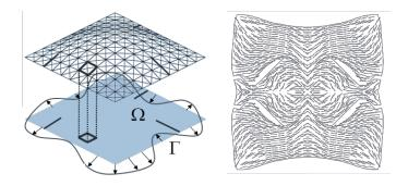
Fig. 1 Deployed CFRP pre-form with optimized fiber orientation
